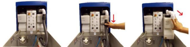
Fig. 14: Remove dirty-water tank
